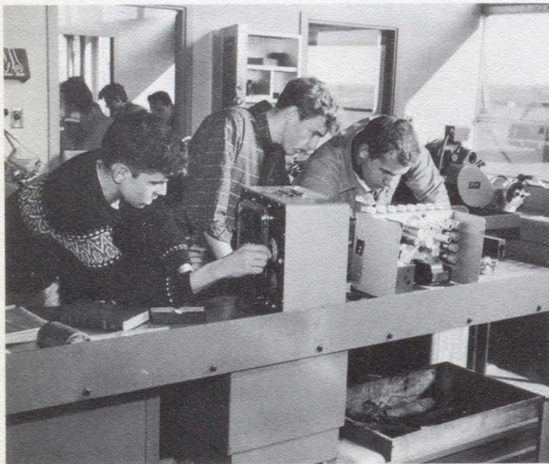
Repairing various equipment is one of the many jobs done by the senior high shop students. Here three boys are using a vacuum volt meter to check an amplifier which has been overheating.
